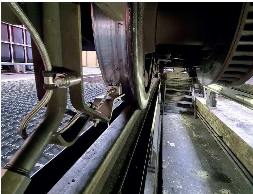
An onboard spraying unit, with the nozzle set to apply top-of-rail conditioning product to the wheel tread.
