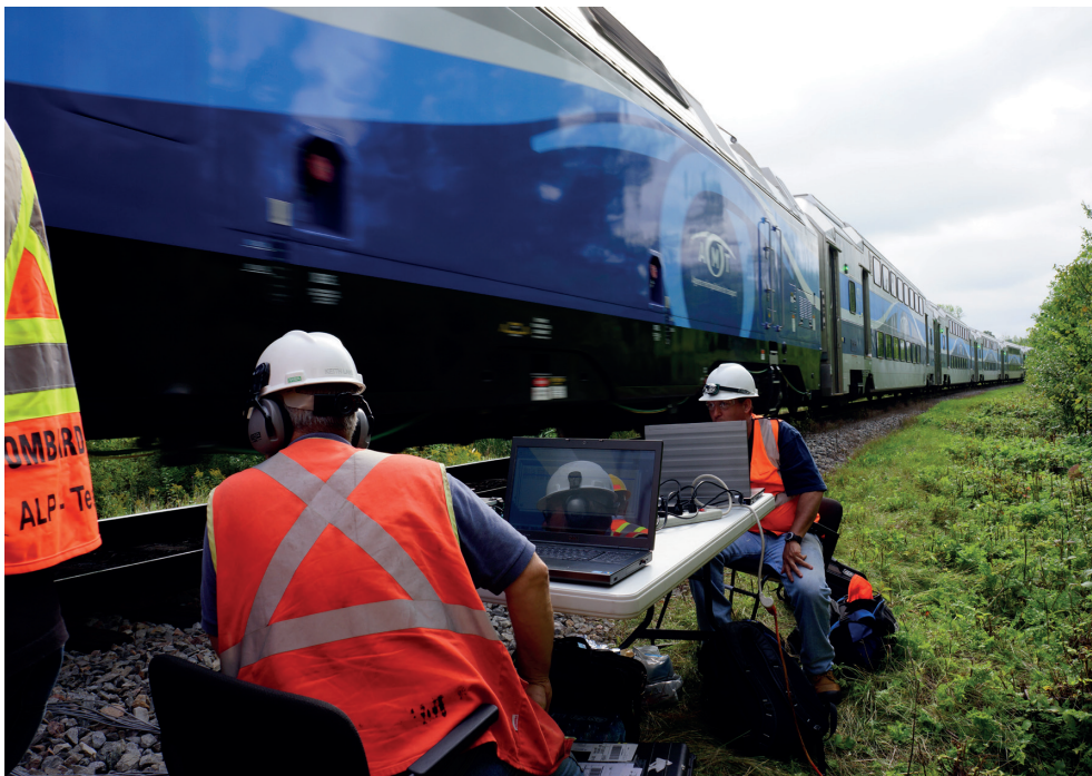
Field testing to assess the impact of friction management products on braking performance.
