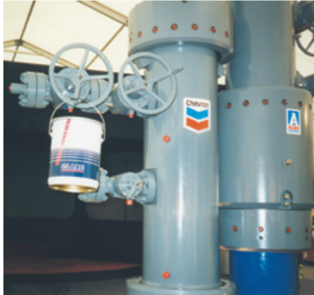
3. Subsea production tree - gate valves
