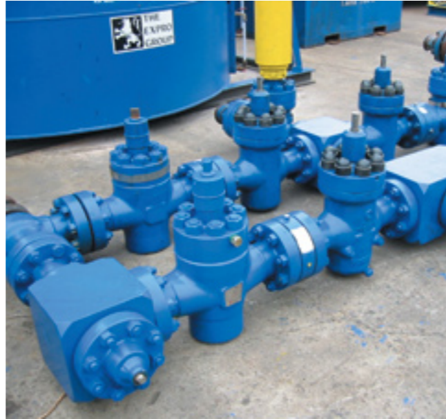
6. Heat exchanger - gate valves
